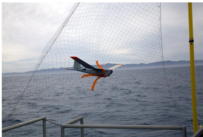
Figure 2. Autonomous net recovery of Puma AE in 2015 on NOAA R/V Shearwater.
