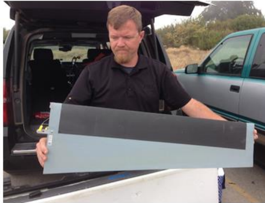
Figure 7. Nano-tube integrated onto airfoil leading edge.
